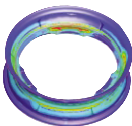
Stresses due to welding and in-service loading
